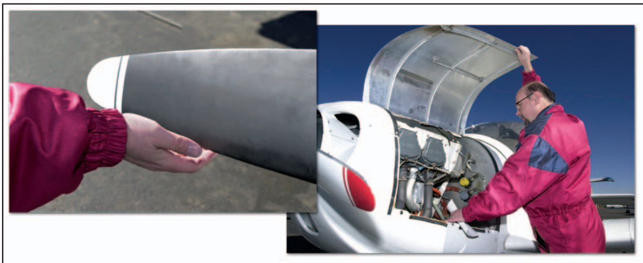
Figure 2-8. Check the propeller and inside the cowling.
