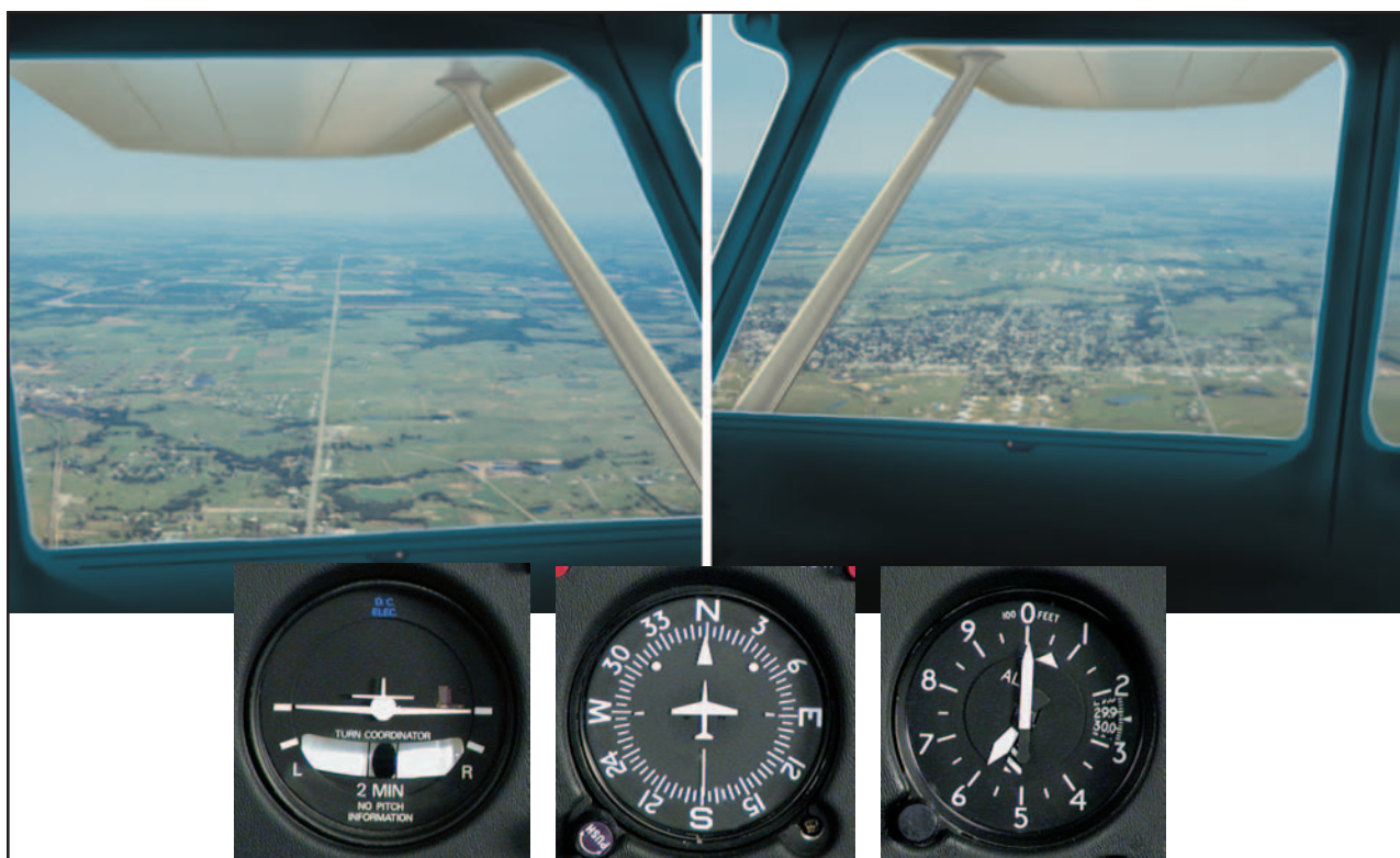
Figure 3-4. Wingtip reference for straight-and-level flight.
