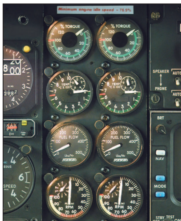
Figure 14-4. Powerplant instrumentation—fixed shaft turboprop engine.
