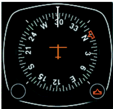
Figure 3-30. The heading indicator is not north-seeking, but must be set to agree with the magnetic compass.
