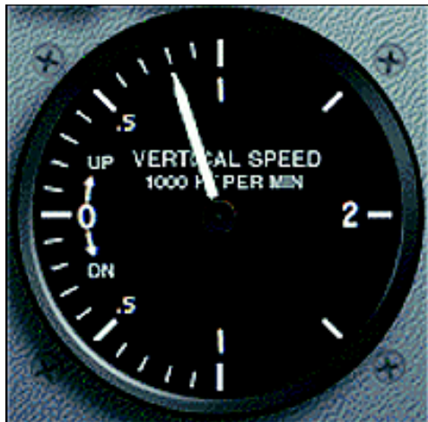
Figure 3-14. Vertical speed indicator shows the rate of climb or descent in thousands of feet per minute.
