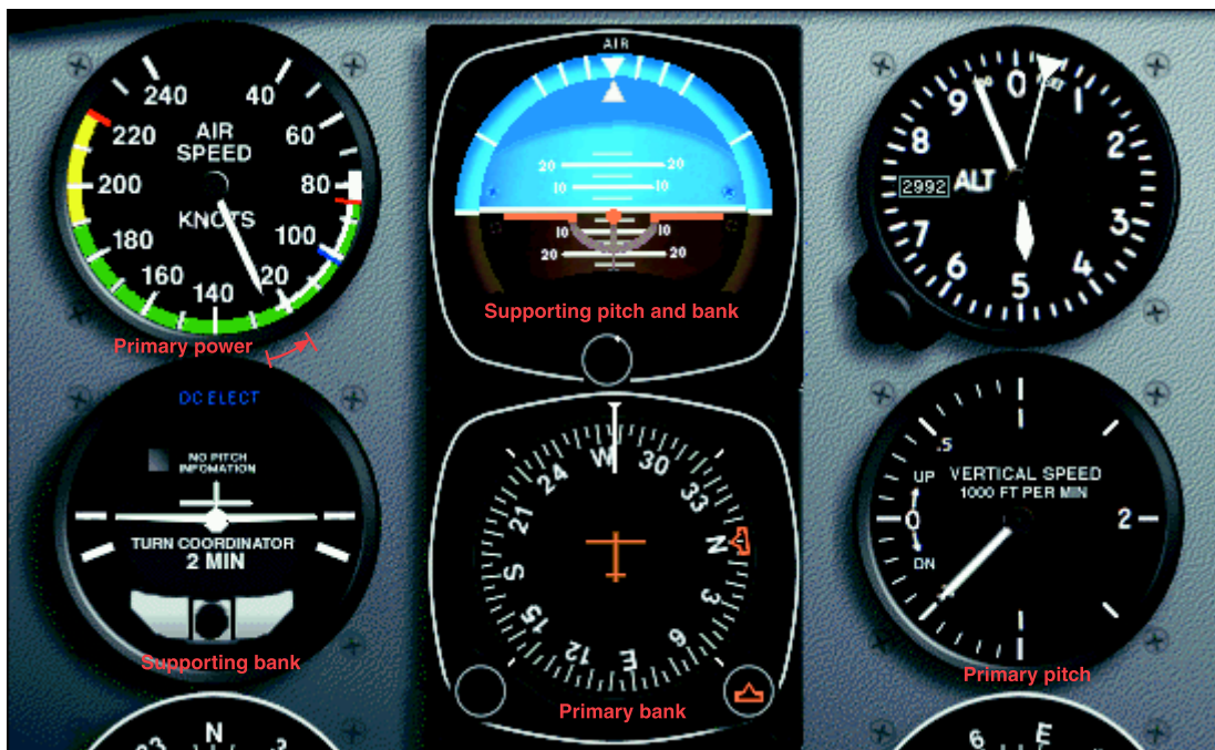
Figure 5-30. Constant airspeed descent, airspeed high—reduce power.
