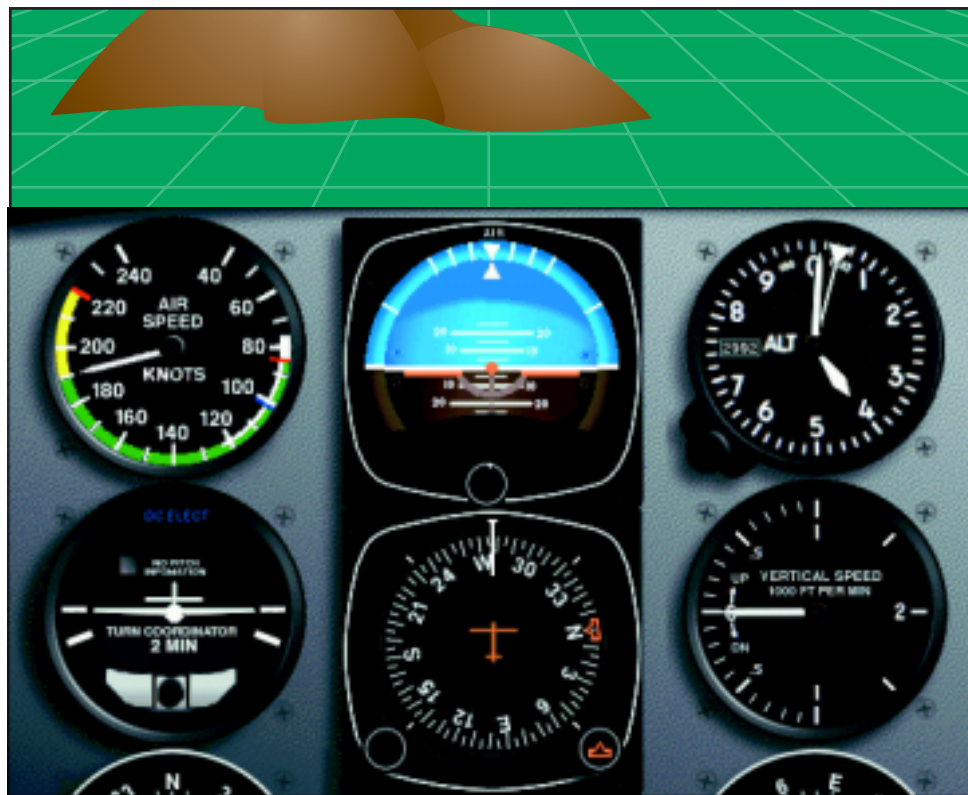
Figure 5-2. Pitch attitude and airspeed in level flight, fast cruise speed.
