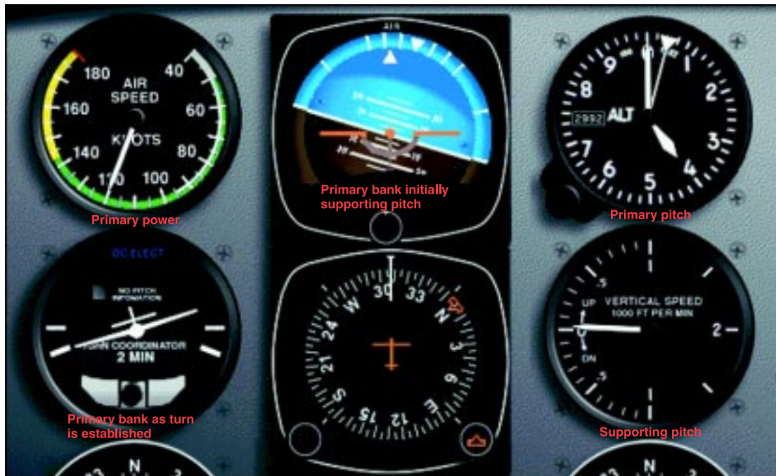
Figure 5-33. Standard-rate turn, constant airspeed.
