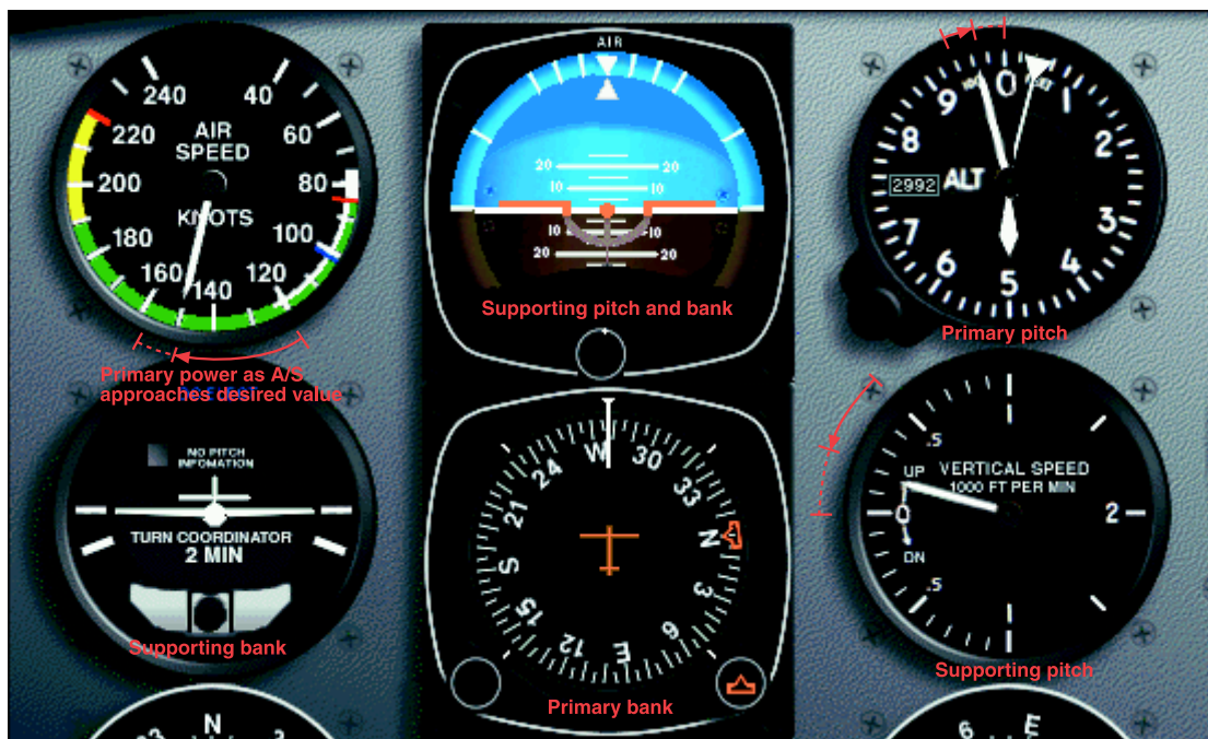
Figure 5-29. Level-off at cruising speed.
