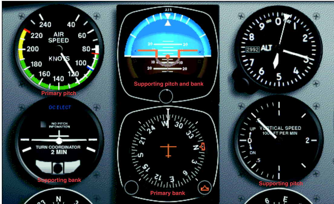
Figure 5-26. Stabilized climb at constant airspeed.
