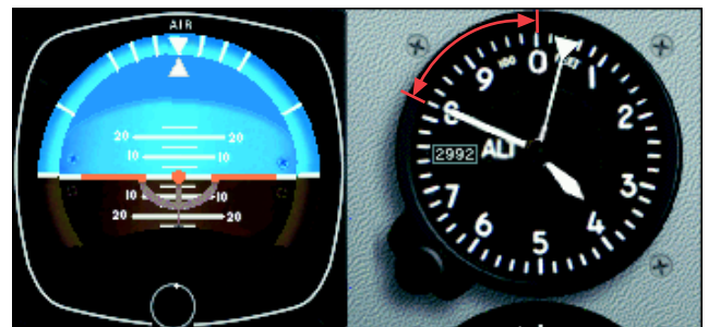
Figure 5-11. Altitude error, greater than 100 feet.
