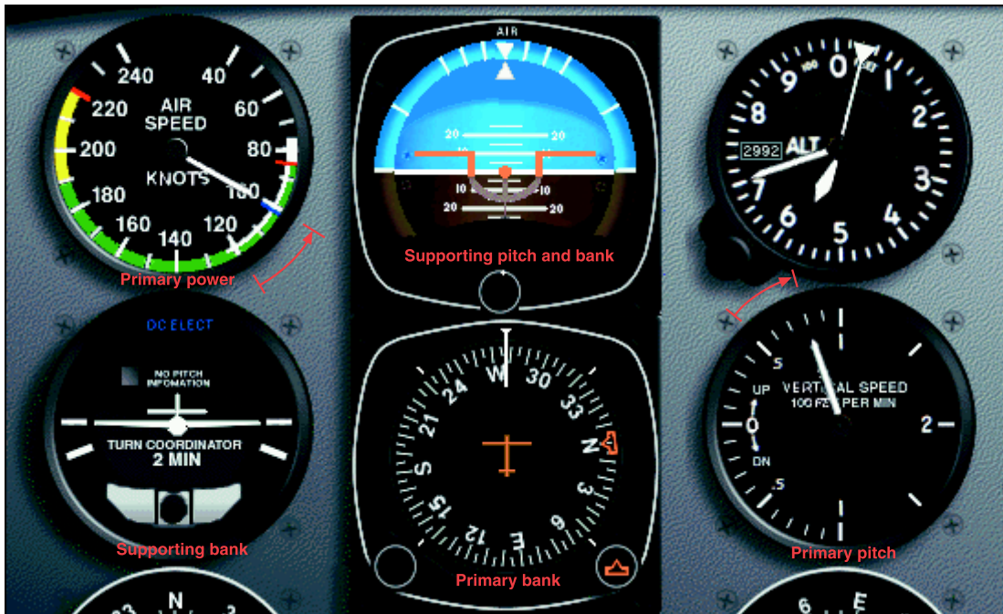
Figure 5-28. Airspeed low and vertical speed high—reduce pitch.
