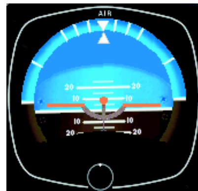
Figure 5-5. Pitch correction for level flight, two-bar width.
