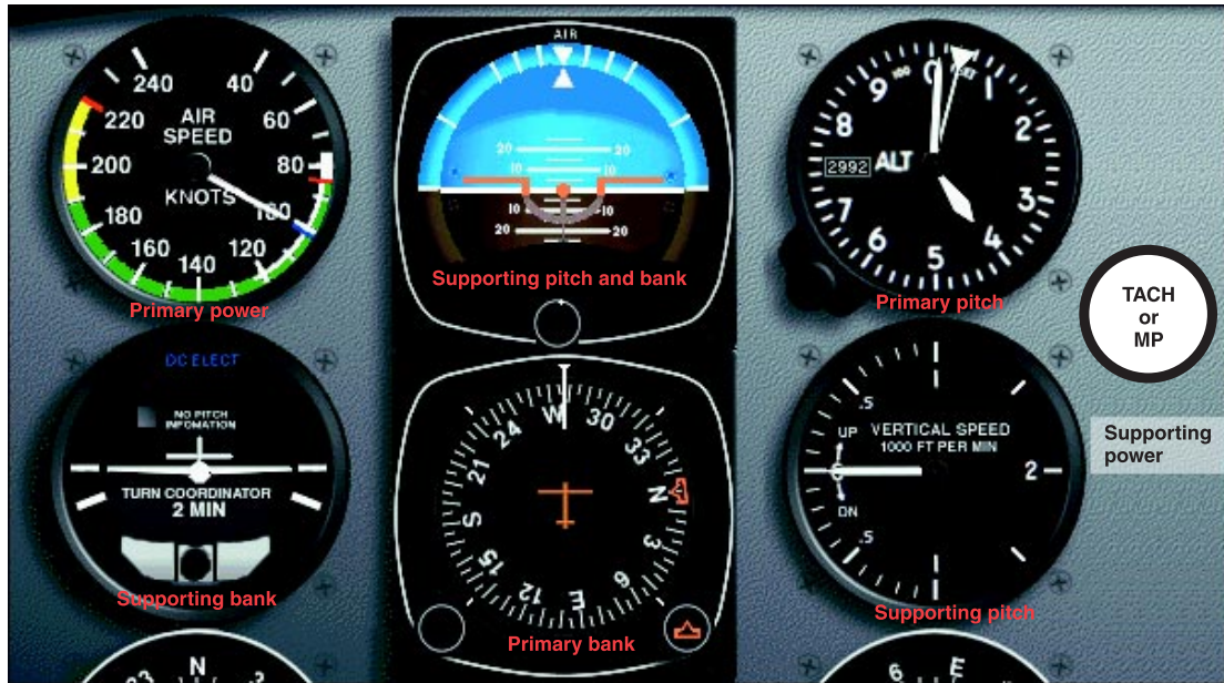
Figure 5-24. Straight-and-level flight (reduced airspeed stabilized).
