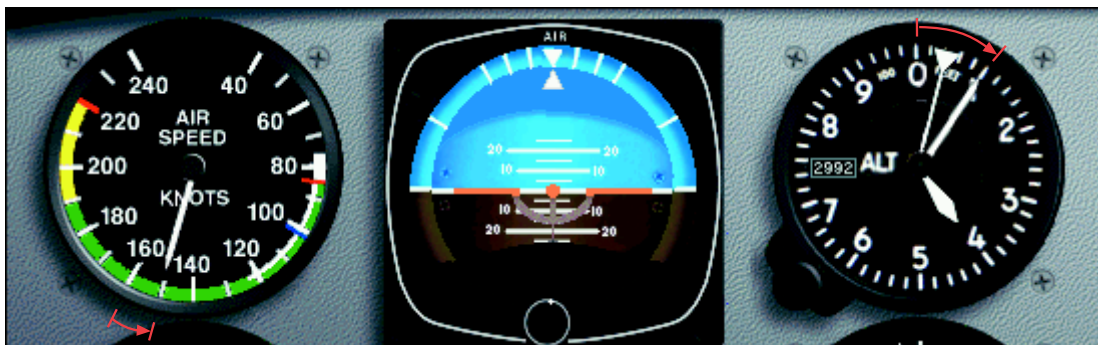
Figure 5-20. Airspeed low and altitude high (lower pitch).
