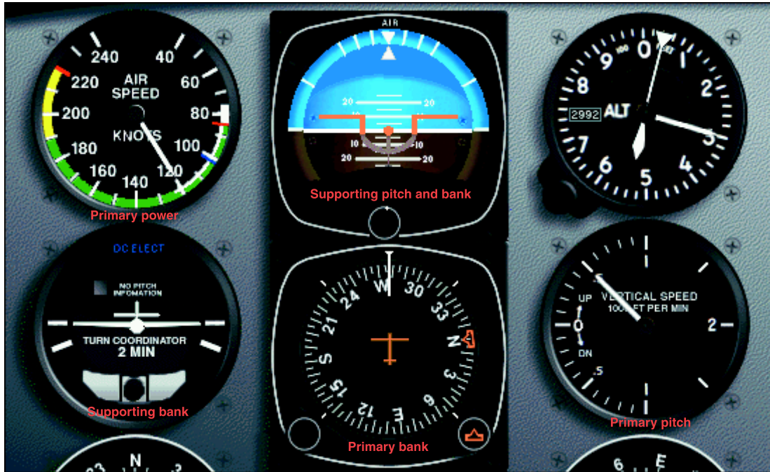
Figure 5-27. Stabilized climb at constant rate.
