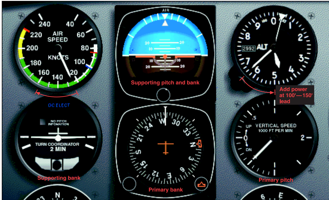
Figure 5-31. Level-off airspeed higher than descent airspeed.
