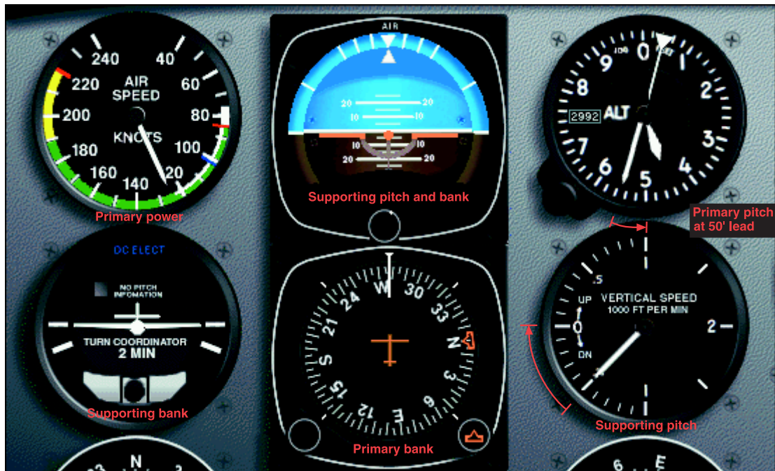
Figure 5-32. Level-off at descent airspeed.
