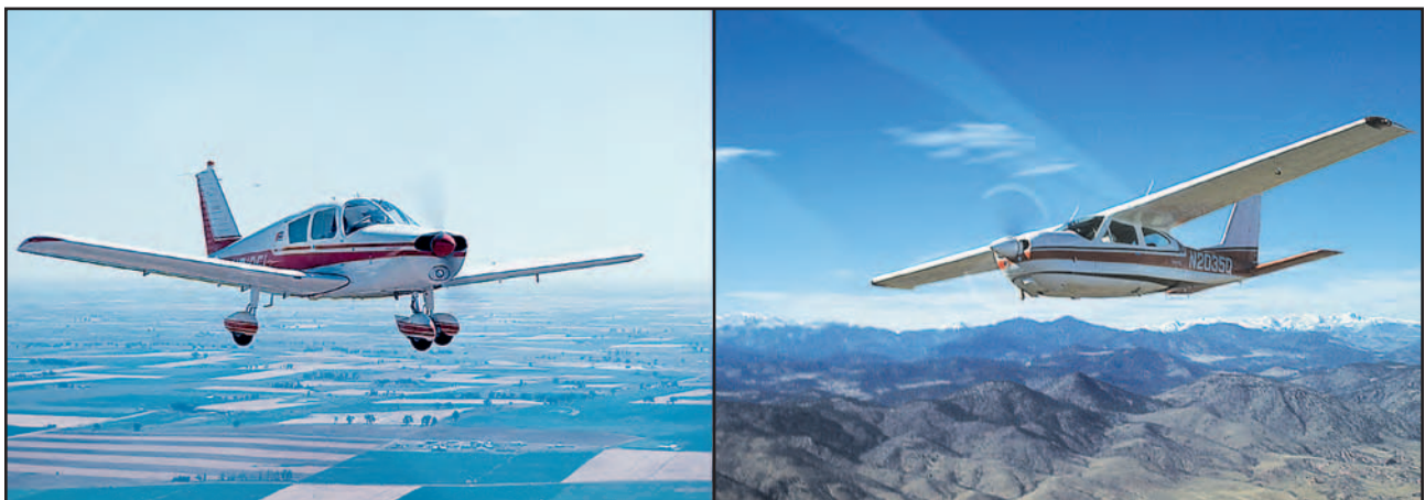
Figure 5-28. Fixed and retractable gear airplanes.
