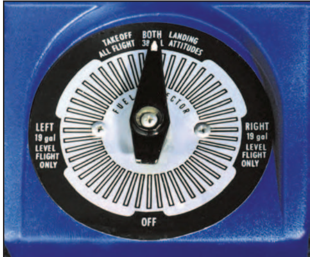
Figure 5-16. Fuel selector valve.
